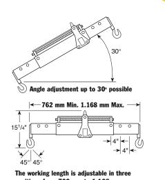
The working length is adjustable in thre positions from 762 mm to 1.168 mm. Maximum chain angle is 45°.
