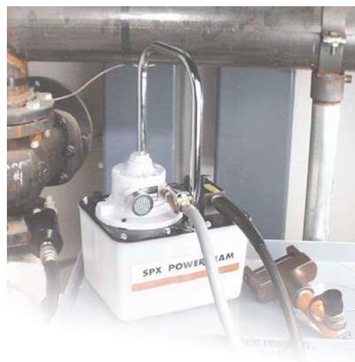
The PA17 used with a flange spreader
