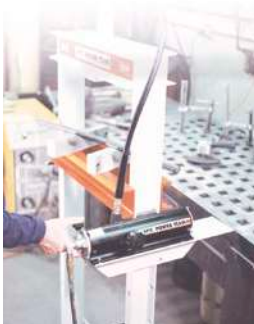
PA9H Hand Control Pump as used in a straightening press.
