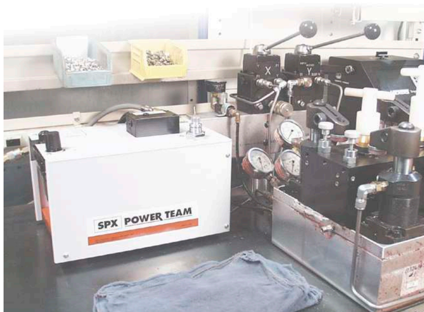
The PA60 used in a workholding environment.
