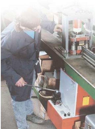
Hydraulic Machine Press Operation.
